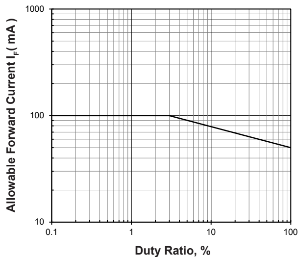
Allowable Forward Current Vs Duty Ratio
