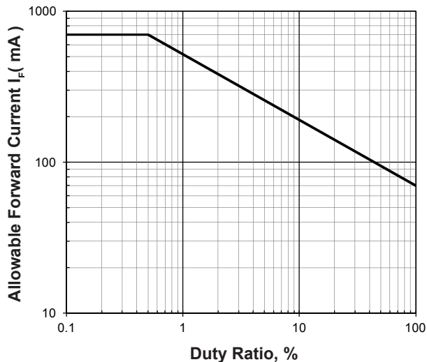
Allowable Forward Current Vs Duty Ratio
