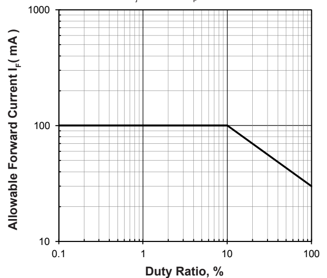
Allowable Forward Current Vs Duty Ratio
