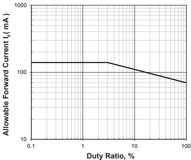
Allowable Forward Current Vs Duty Ratio
